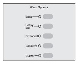
Press the button for the wash options you would like to select. The indicator light for the respective option will illuminate.
